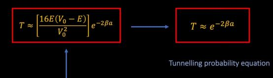
$$T = \frac{|C|^2}{|A|^2} = \frac{C^*C}{A^*A} = \left[\frac{16k^2\beta^2}{(\beta^2 + k^2)^2}\right]e^{-2\beta a} \qquad k = \frac{\sqrt{2mE}}{\hbar} \qquad \beta = \frac{\sqrt{2m(V_0 - E)}}{\hbar}$$
