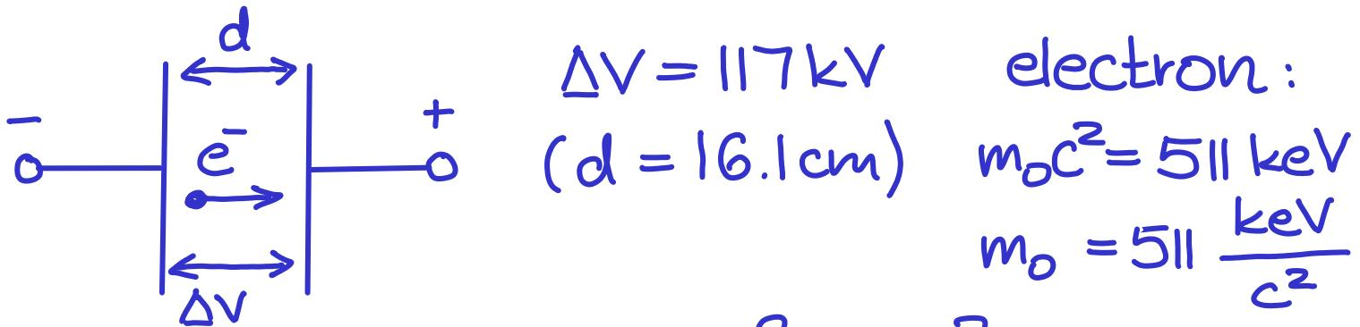
$$W = e \cdot \Delta V = KE \quad \begin{array}{l} \beta_{\text{class}} = ? \\ \beta_{\text{rel}} = ? \end{array}$$
