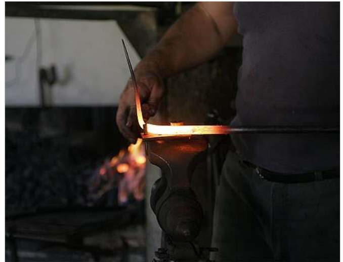
Blacksmiths judge workpiece temperatures by the colour of the glow. [7]
