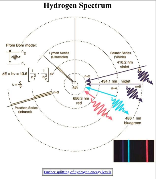
This spectrum was produced by exciting a glass tube of hydrogen gas with about 5000 volts from a transformer. It was viewed through a diffraction grating with 600 lines/mm. The colors cannot be expected to be accurate because of differences in display devices.
