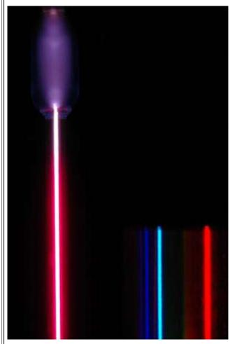
At left is a hydrogen spectral tube excited by a 5000 volt transformer. The three prominent hydrogen lines are shown at the right of the image through a 600 lines/mm diffraction grating.
