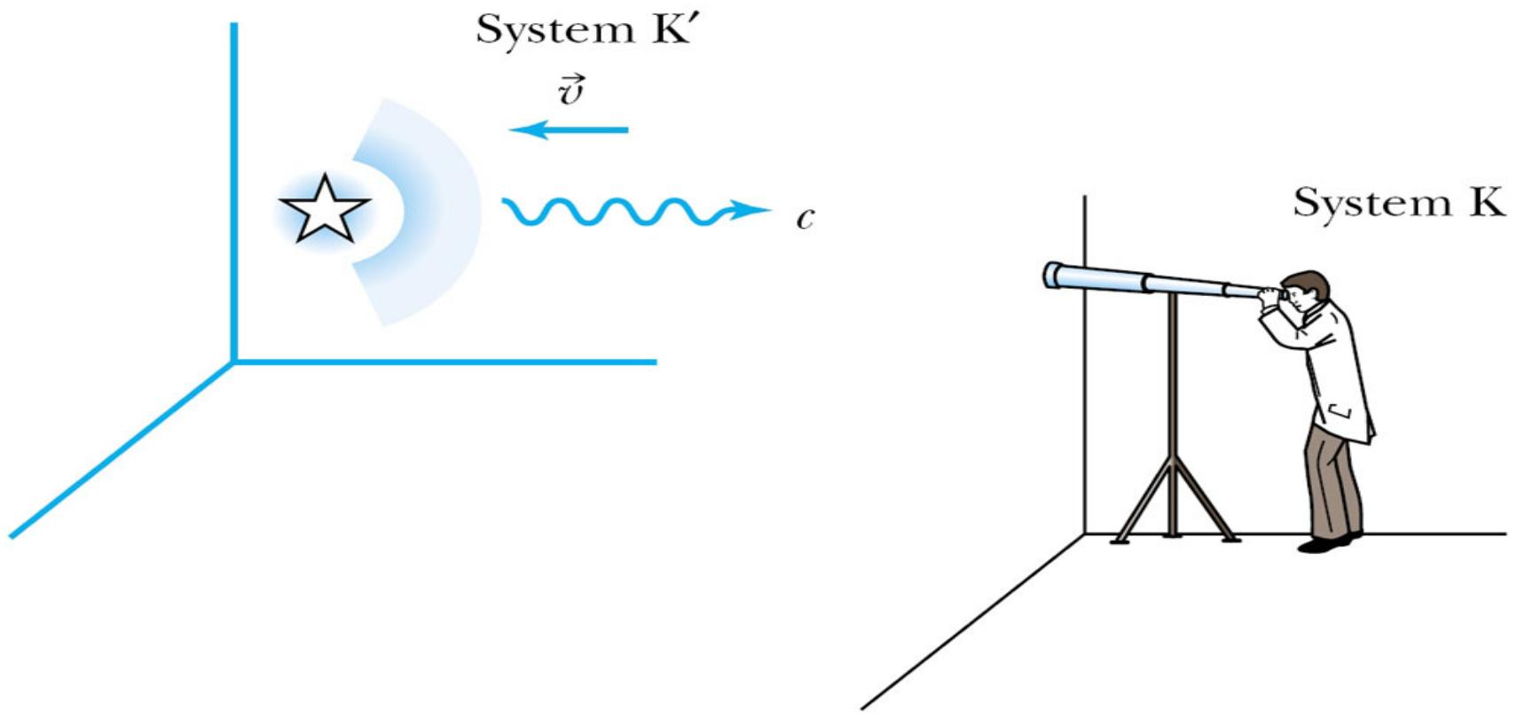
Suppose an observer in system K views light from a star that is receding with velocity  $v$ . In a time  $T$ , the length of the wave train is
