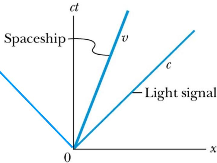
In the  $x$ - $ct$  plane, we can plot the trajectories of objects. Light signals follow a 45 degree line since  $\Delta s^2 = 0$ .
