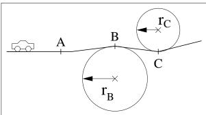
The radii of curvatures at  ${\bf B}$  and  ${\bf C}$  are:  ${\bf r}_{\rm B}=135$  m and  ${\bf r}_{\rm C}=125$  m. Calculate the normal force exerted by the road on the car at point  ${\bf A}$ .
