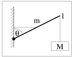
2 pt The boom makes an angle of  $\theta = 51.4^{\circ}$  with the vertical wall. Calculate the tension in the vertical rope. (in N)
