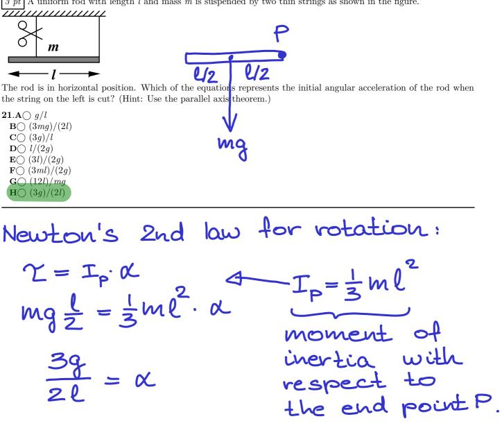
3 pt A uniform rod with length l and mass m is suspended by two thin strings as shown in the figure.
