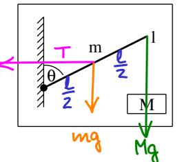
2 pt The boom makes an angle of  $\theta = 51.4^{\circ}$  with the vertical wall. Calculate the tension in the vertical rope. (in N)
