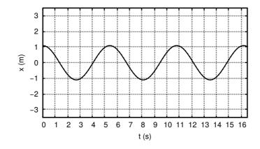
The graph shows the x-displacement as a function of time for a particular object undergoing simple harmonic motion.
