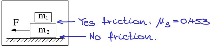
The coefficient of static friction between the two blocks is  $\mu_s = 0.453$ . The friction between the bottom block and the horizontal surface is negligible.
