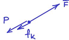
The angle of the incline is  $\theta = 39.7^{\circ}$ . The object is observed to move at a constant velocity of 2.13 m/s up on the incline. Calculate the magnitude of the frictional force acting on the object.
