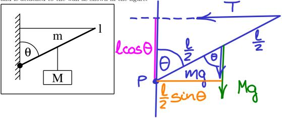
3 pt The boom makes an angle of  $\theta = 62.1^{\circ}$  with the vertical wall. Calculate the tension in the vertical rope.
