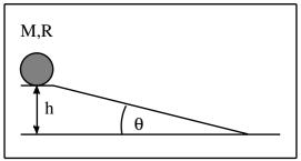
The height of the incline is h = 1.87 m, and the angle of the incline is  $\theta = 10.9^{\circ}$ . The cylinder is rolled over the edge very slowly. Then it rolls down to the bottom of the incline without slipping. What is the final speed of the cylinder? (in m/s)
