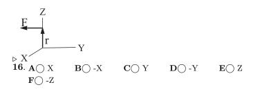
10 pt A small mass M attached to a string slides in a circle (Y) on a frictionless horizontal table, with the force **F** providing the necessary tension (see figure). The force is then decreased slowly and then maintained constant when M travels around in circle (X). The radius of circle (X) is twice the radius of circle (Y).
