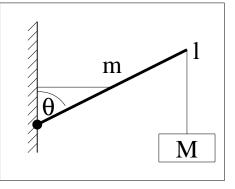
2 pt The boom makes an angle of  $\theta = 65.0^{\circ}$  with the vertical wall. Calculate the tension in the vertical rope. (in N)
