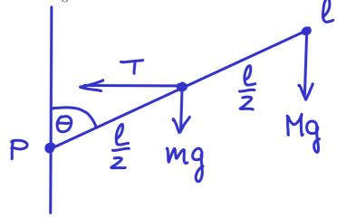
3 pt The boom makes an angle of  $\theta = 51.6^{\circ}$  with the vertical wall. Calculate the tension in the vertical rope.
