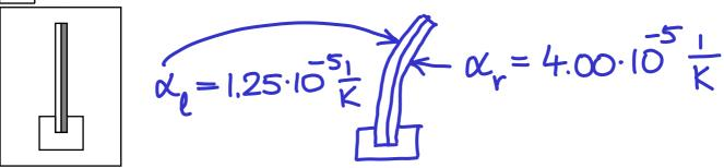
The metal on the left has a coefficient of linear heat expansion of  $\alpha_{\rm left} = 1.25 \times 10^{-5}$  1/K, the metal on the right has  $\alpha_{\rm right} = 4.00 \times 10^{-5}$  1/K. When the strip is cooled, it will ... (complete the sentence)
