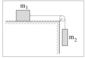
The pulley is massless and frictionless. The system is observed to move with constant speed. Determine  $\mu_k$ , the coefficient of kinetic friction between mass  $m_1$  and the surface of the table.
