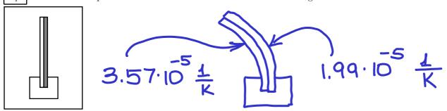
3 pt A bimetallic strip is held fixed at the bottom end as shown in the figure.
