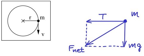
2 pt When it is at the location shown, (mid-height), its speed is v = 4.13 m/s. Determine the tension in the rope. (in N)
