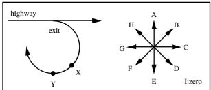
3 pt The driver slows the car down to the posted speed limit, enters the exit ramp and then maintains a constant speed. When the car is at point **X** on the ramp, which vector best represents the direction of the car's acceleration?
