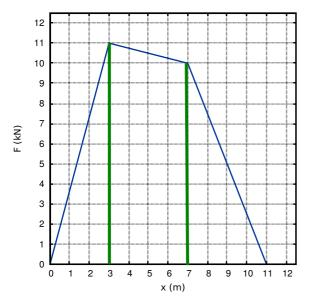
The area under the force vs. displacement function is work. Work divided by time is power.
