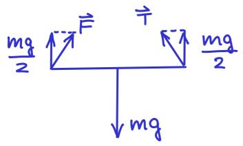
The vertical component of the force F is half the weight:  $F_y = \frac{mg}{-g}$ 27.0 · 9.81 = 132N
